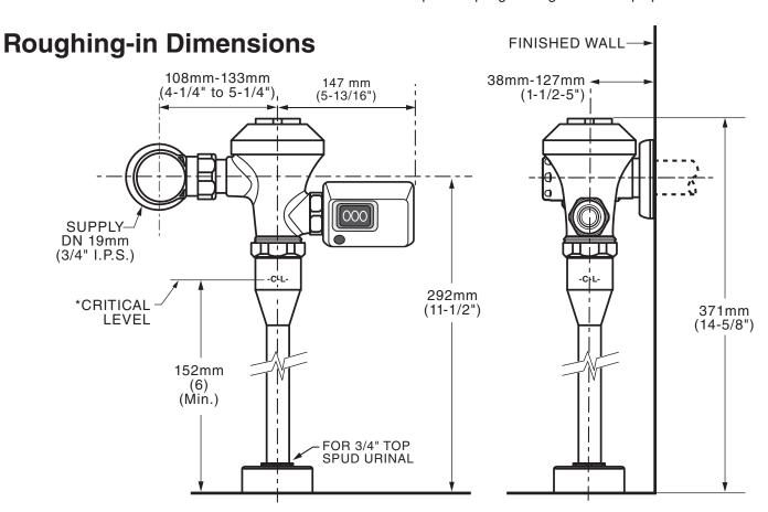
\*Note: The Critical Line (-C-L-) on Vacuum Breaker must typically be a minimum of 6" (152 mm) above fixture. Consult Codes for details.
